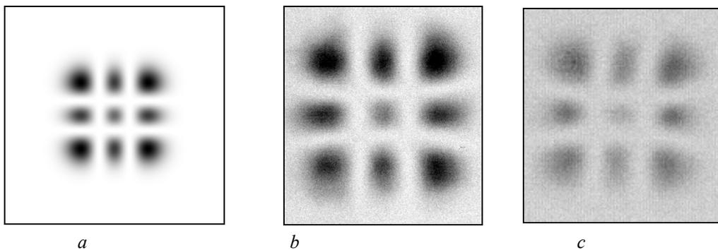
Fig. 5. Intensity distribution in the cross-section of unimodal beam (Gauss-Hermite  $(2,2)$ ): a) result of computer simulation, b),c) – intensity distributions measured in different focal planes of the lens L2.
