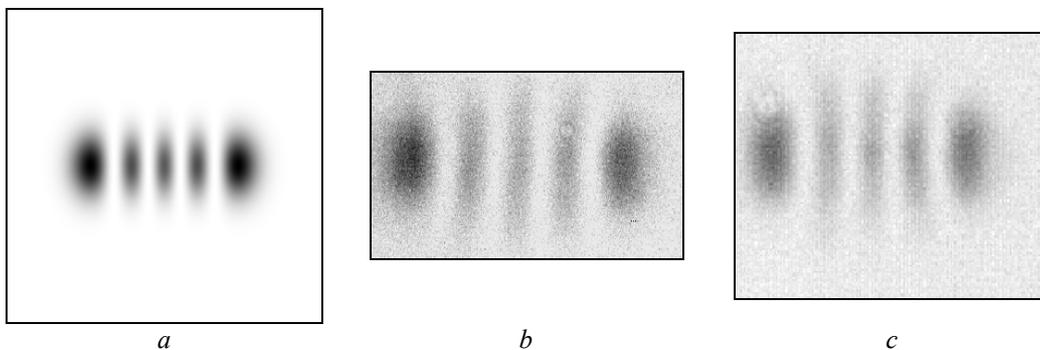
Fig. 6. Intensity distribution in the cross-section of unimodal beam (Gauss-Hermite  $(4,0)$ ): a) result of computer simulation, b),c) – intensity distributions measured in different focal planes of the lens L2.
