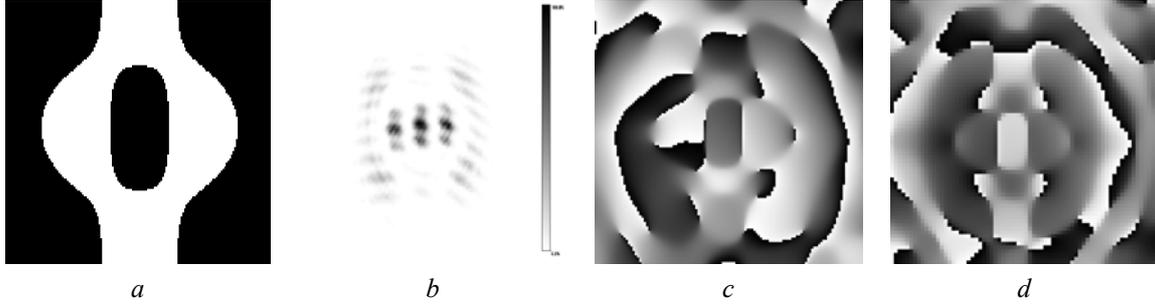
Fig. 7. Phase distribution in the cross-section of two-modal beam (Gaussian-Hermite (4,0)+(2,2)) with intermodal phase shift value  $\Delta\varphi=0$ :
