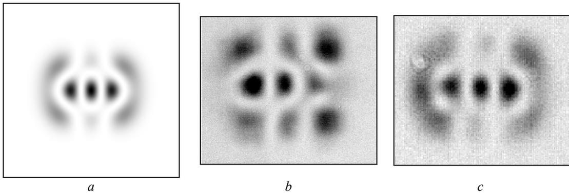
Fig. 3. Intensity distribution in the cross-section of two-modal beam (Gauss-Hermite  $(4,0)+(2,2)$ ) with intermodal phase shift value  $\Delta\varphi=0$ : a) result of computer simulation, b),c) – intensity distributions measured in different focal planes of the lens L2
