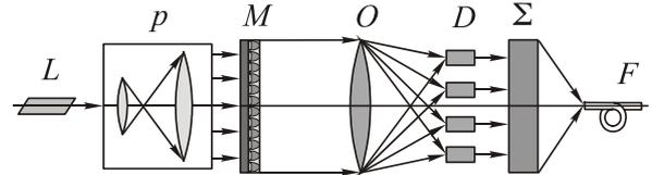
Fig. 8. General scheme of a multichannel waveguide telecommunication system:  $L$  - laser light source,  $P$  - collimator,  $M$  - MODAN,  $O$  - Fourier stage,  $D$  - set of modulators,  $F$  - ideal parabolic index fiber.
