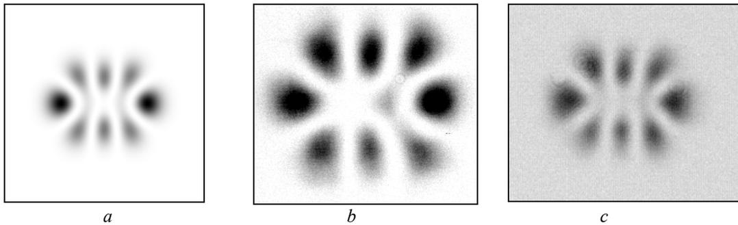
Fig. 4. Intensity distribution in the cross-section of two-modal beam (Gauss-Hermite  $(4,0)+(2,2)$ ) with intermodal phase shift value  $\Delta\varphi=\pi$ : a) result of computer simulation, b), c) – intensity distributions measured in different focal planes of the lens L2.
