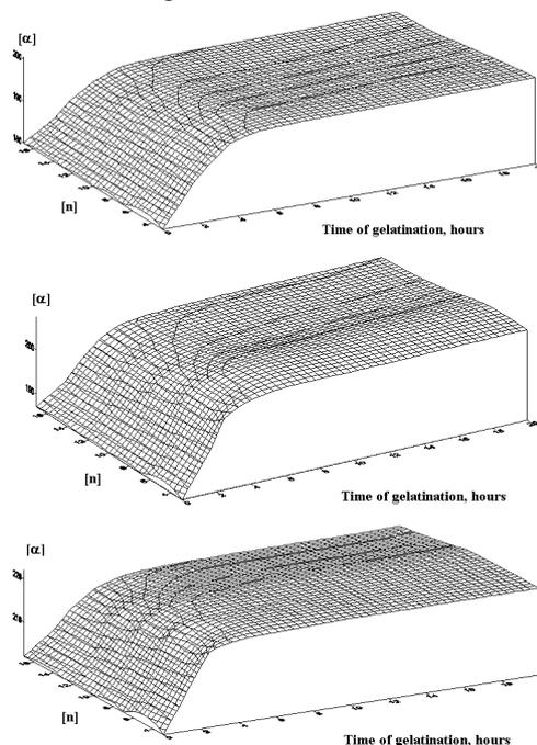
Fig. 1. The change of kinetics of the normalized optical rotation angle at  $20^\circ\text{C}$  for SD DG layers with the gelatin concentration: a) 3 %, b) 7 %, c) 10 %.  $[n]$  = glycerol concentration.
