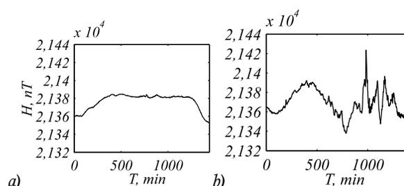
Fig. 1.  $H$ -components of the magnetic field of the Earth: a) quiet diurnal variation; b) perturbed diurnal variation
