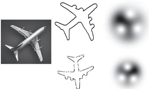
Fig. 5. From left to right: the aircraft initial image, the outlined boundary contour, the intensity of the generated spiral beam
