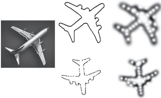
Fig. 4. From left to right: the aircraft initial image, the outlined boundary contour, the intensity of the generated spiral beam
