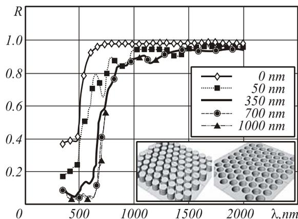
Figure 2. Calculated spectral reflectivity curves,  $R(\lambda)$ . Each pictured curve corresponds with a 2D-Au-SWS-1 and a 2D-Au-SWS-2, whereas the pillar height of the first type structure is equal to the hole depth of the second one. Each curve corresponds with a specific feature height/depth
