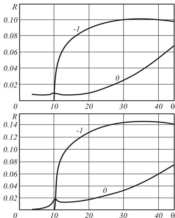
Figure 1. In this figure, reflectivity curves of single diffraction orders produced by a beam of wavelength 550nm are reported here for two particular square symmetry 2D-SWS of tungsten, and against the beam angle of incidence. Reflectivity is defined like the percentage of the incident beam energy reflected by the structure.
