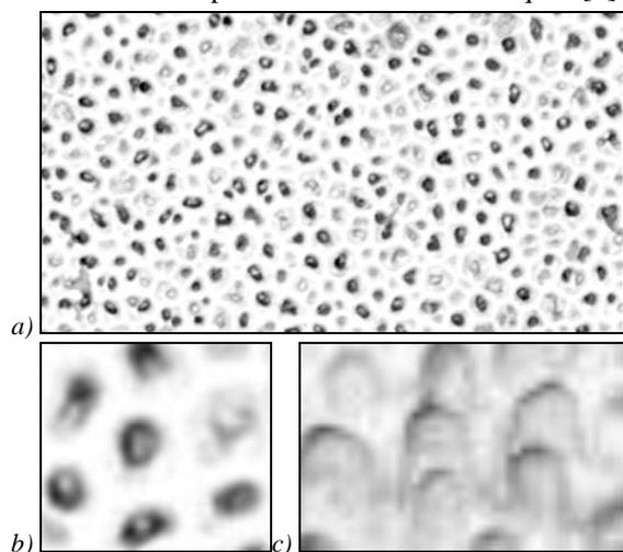
Figure 3. SEM images of the fabricated 2D-Au-SWS. The images show a rhombic symmetry 2D-Au-SWS made up of pillars 700nm high, spaced about 150nm from each other and of 250nm diameter circular base.
