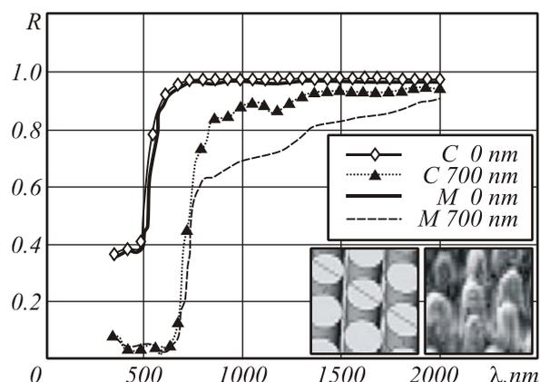
Figure 4. Spectral reflectivity curves. C-curves represent the reflectivity calculated by 7<sup>th</sup> order-RCWA, while M-ones are measurements. -The diamond marked curve is the calculated reflectivity of a gold flat surface, while the non-marked bold line is the relative measured curve. - Line marked with triangles shows the calculated reflectivity of a 2D-Au-SWS-1 made of 700nm high pillar. - The dashed line curve is the measured reflectivity of the 2D-Au-SWS prototyped
